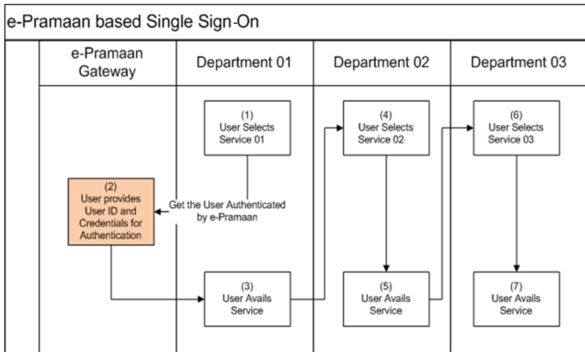
Figure 1: e-Pramaan based single sign-on
